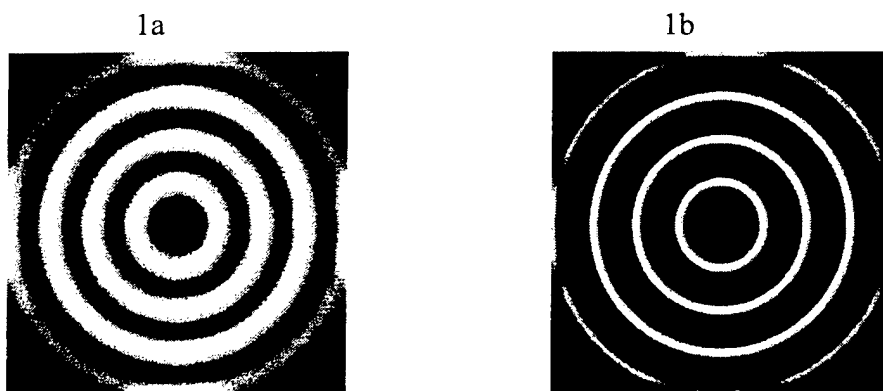
Figs. 2a and 2b: Blurred “Circles” image and its restoration by ML algorithm
