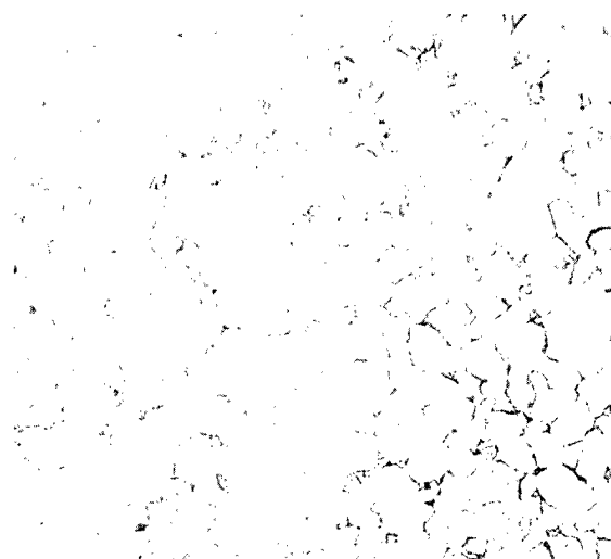
Figure 3. Th-5 W /o Pu. Cold reduced 90% and heat treated one minute at 650°C. Etch: 100cc ethyl alcohol, 10cc perchloric acid 2 sec. at 40v. 400X. PL98.
