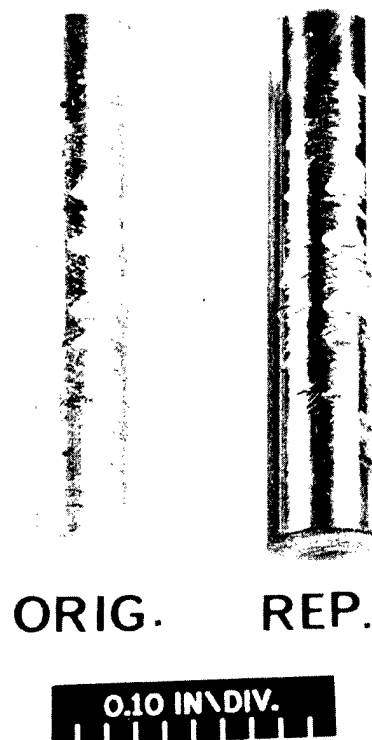
Figure 2. Comparison of Original Specimen Which Was Replicated in Figure 1 and Aluminum Shadowed Epoxy Replica Cast from RTV Mold. R-14557.
