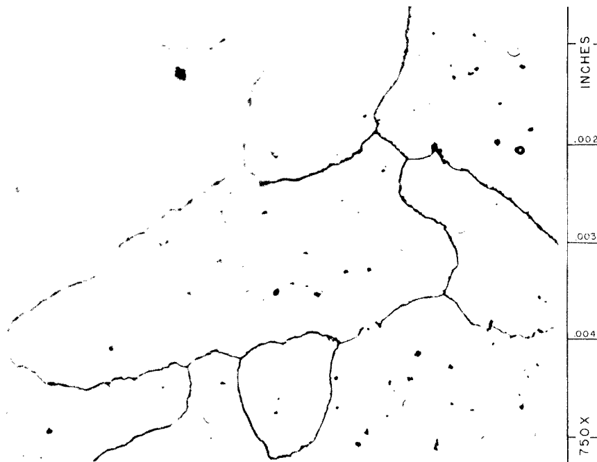
Figure 6. Photomicrograph of Aluminized Replica of Microcrack Found in Rim of MSRE Flange. 100X. Y-47911.
