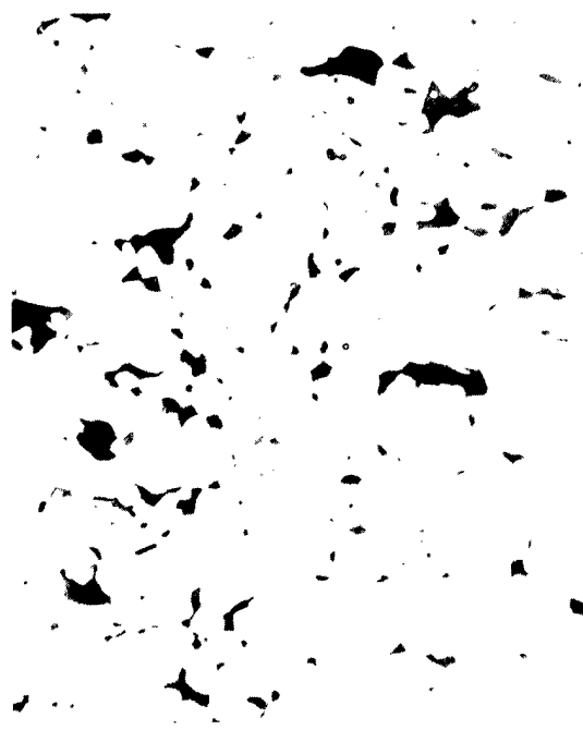
Figure 9. Same Field as Figure 8 after Prolonged Nitric-Acetic-Water Etch. 500X.
