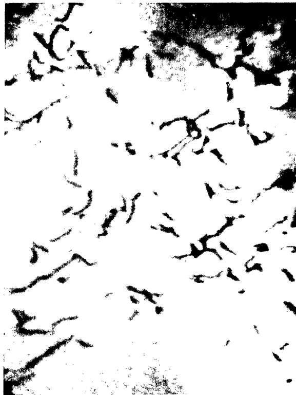
Figure 2. Three Percent Cold Rolled Alpha Uranium. 18,000X.
