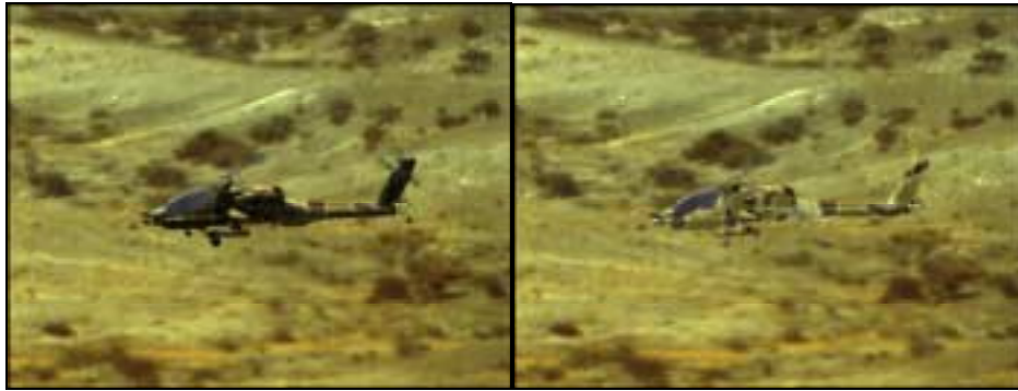
Figure 6. GTV Camouflage Design: (left) Color Matching to Background; (right) Additional Correction for Lighting Intensities (i.e. the shadows on the side and bottom were reduced)
