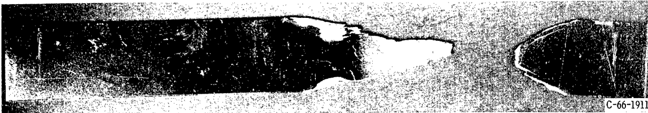
(c) Exposed to hydrogen atmosphere for 1 hour at 2780° F; heating rate, 100° F per minute; cooling rate, 40° F per minute.
