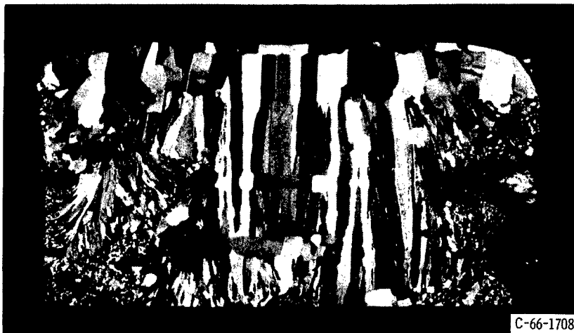
Figure 2. - Longitudinal grain structure of second-melt ingot whose initial composition was tungsten-0.5 weight percent boron. Murakami's etchant, X2.4.
