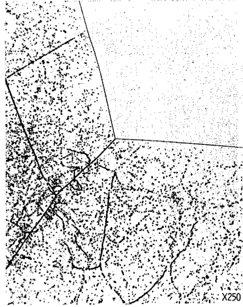
Figure 3. - Transverse cross section and microstructure of unalloyed tungsten after first and second electron-beam melts.
