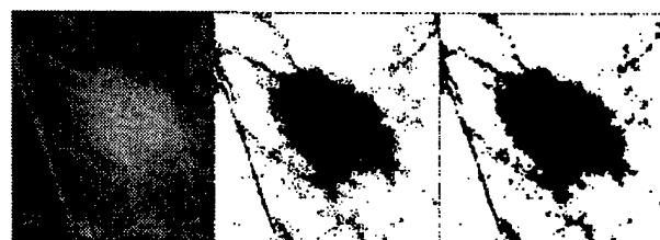
Figure 3. Two-class segmentation results - Example 2: original ROI image (left), and segmentation results using neural network with \lambda = 0 (center) and \lambda = 2 (right).
