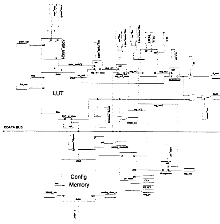
Figure 4: Cell design for the simulated FPGA (includes configuration elements and special logic to allow scanning)
