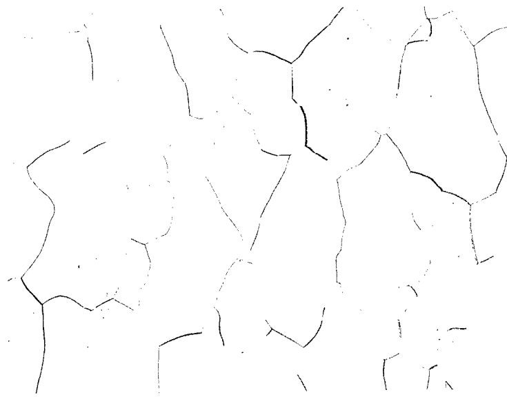
Fig. 14 - Photomicrograph of commercial tungsten. Etched 20% Murakamis, 250X.
