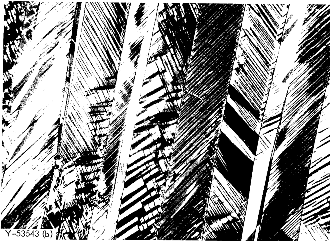
Fig. 10. Arc Cast \text{ThC}_2 Passivated by Immersing 1 min in 1:1 \text{HNO}_3 - \text{H}_2\text{O} . (a) Bright field. (b) Polarized light. 1000 X.
