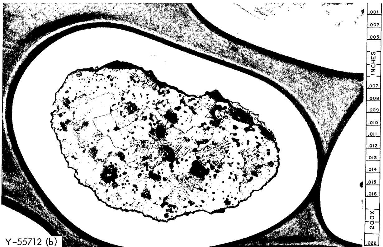
Fig. 4. Pyrolytic Carbon-Coated (Th,U)C_2 Particle of 2.2 Th/U Ratio. (a) Passivated by immersing 30 sec in HNO_3-H_2O . (b) Air etched during vibratory polishing in room atmosphere. 200 X.
