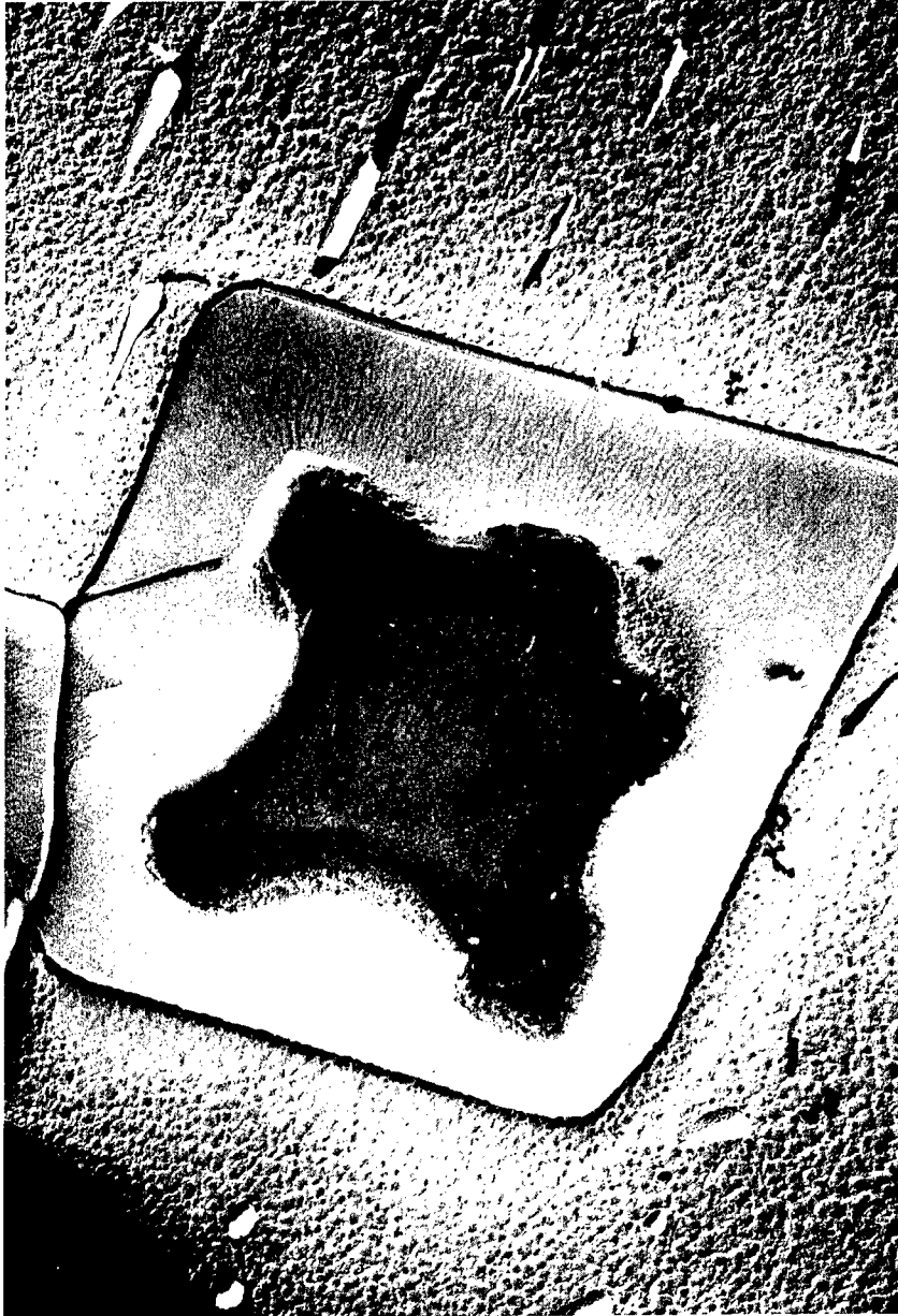
FIGURE 14. LARGE CARBIDE AND SMALL PARTICLES IDENTIFIED AS URANIUM CARBIDE AT EDGE OF INGOT B-85559.
