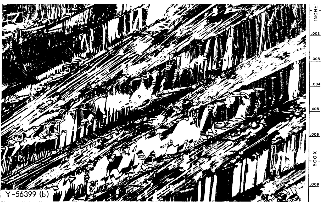
Fig. 6. Arc Cast \text{ThC}_2 Etched by Immersing 45 min in 1:1 \text{HNO}_3\text{-H}_2\text{O} . (a) Bright field. (b) Polarized Tight. 500 X.
