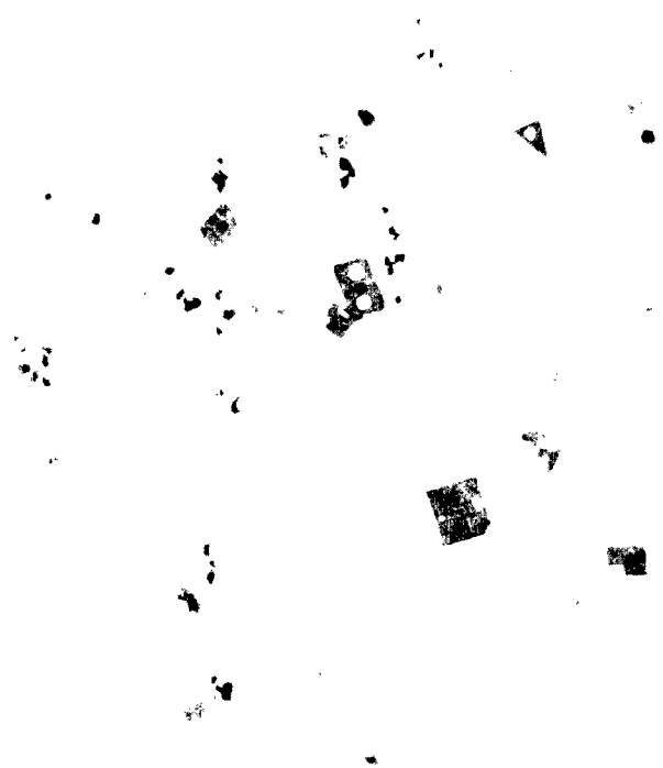
Figure 1 Inclusions in Uranium Metal, Bright Field (100X)
