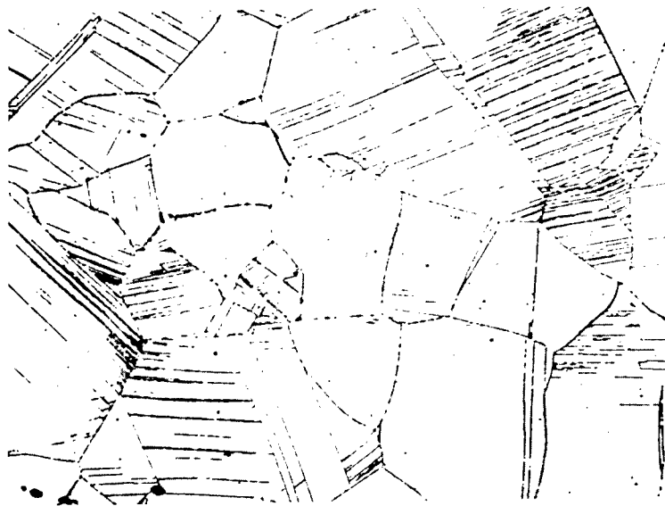
Figure 16. Type 304 Stainless Steel, Sensitized, Polished 2 Hours under a 125-Gram Load. Etched Electrolytically in 10% Oxalic Acid.
