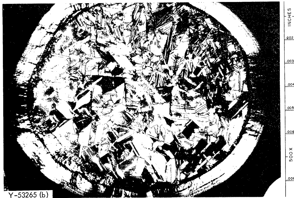
Fig. 7. Pyrolytic Carbon-Coated \text{ThC}_2 Particle Passivated by Immersing 1 min in 1:1 \text{HNO}_3\text{-H}_2\text{O} . (a) Bright field. (b) Polarized light. 500 X.
