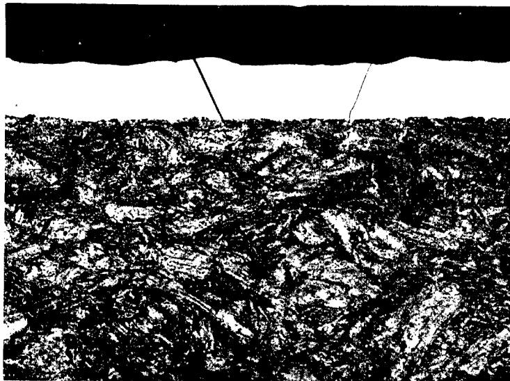
Fig. 9 - Photomicrograph of the same specimen as Fig. 8 prepared using hydrogen peroxide. As-polished, 250X.
