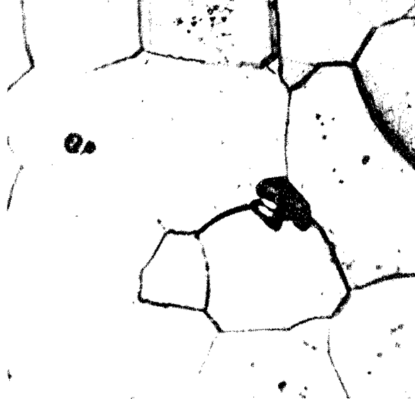
Sample No. B-954 Mag.: 500 X Ident. T-180-N Etch: Murakamis Remarks: As-sintered 4 hrs at 2,400° C; ASTM grain size No. 5-6; 99.5-pct of theoretical density.
