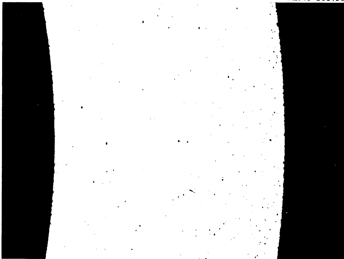
Fig. 6. Complete Decarburization Across Wall of 1-in.-OD, 0.122-in.-Wall Croloy 9M Tubing Exposed to NaK at 1385°F for 5133 hr. 39X
