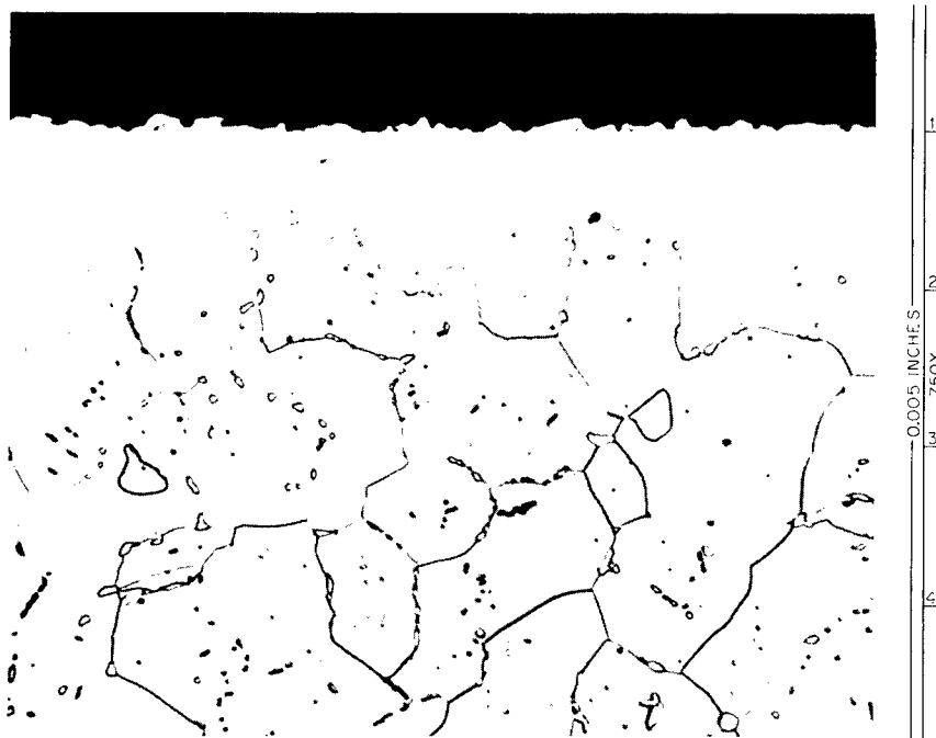
Fig. 3.12. Decarburized Croloy 9M Exposed to NaK at 1242°F for 5133 hr. Specimen No. 10, loop 5-5.
