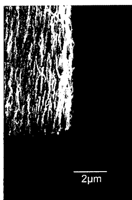
Figure 3(a). Using a C_2H_2 ratio of 15%, etching of the unpatterned Si areas is observed.
