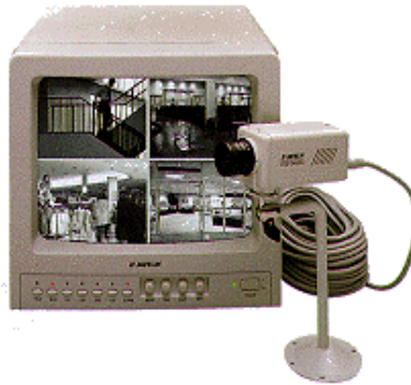
Analog CCTV surveillance system.
