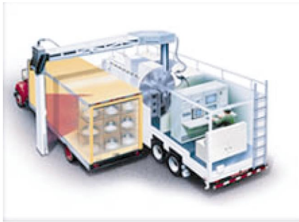
X-ray inspection of a truck.
