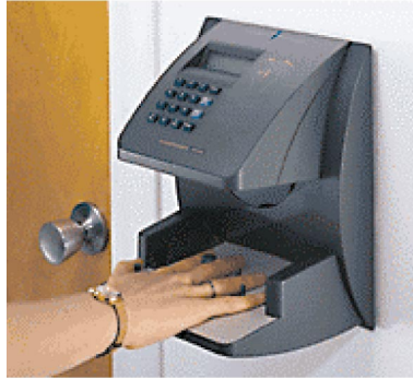
Access control terminal. Source: Recognition Systems, Inc.
