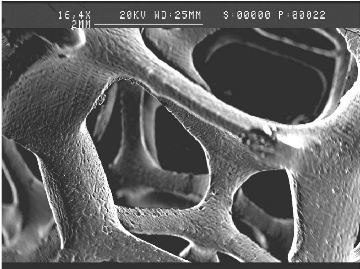
Figure 27 SEM Image of 10 PPI Aluminum Foam Before Compression
