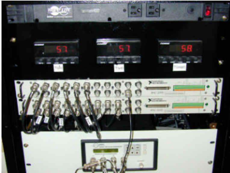
Figure 9. BNC 500 Pulse Generator and Data Acquisition Break-Out Panel
