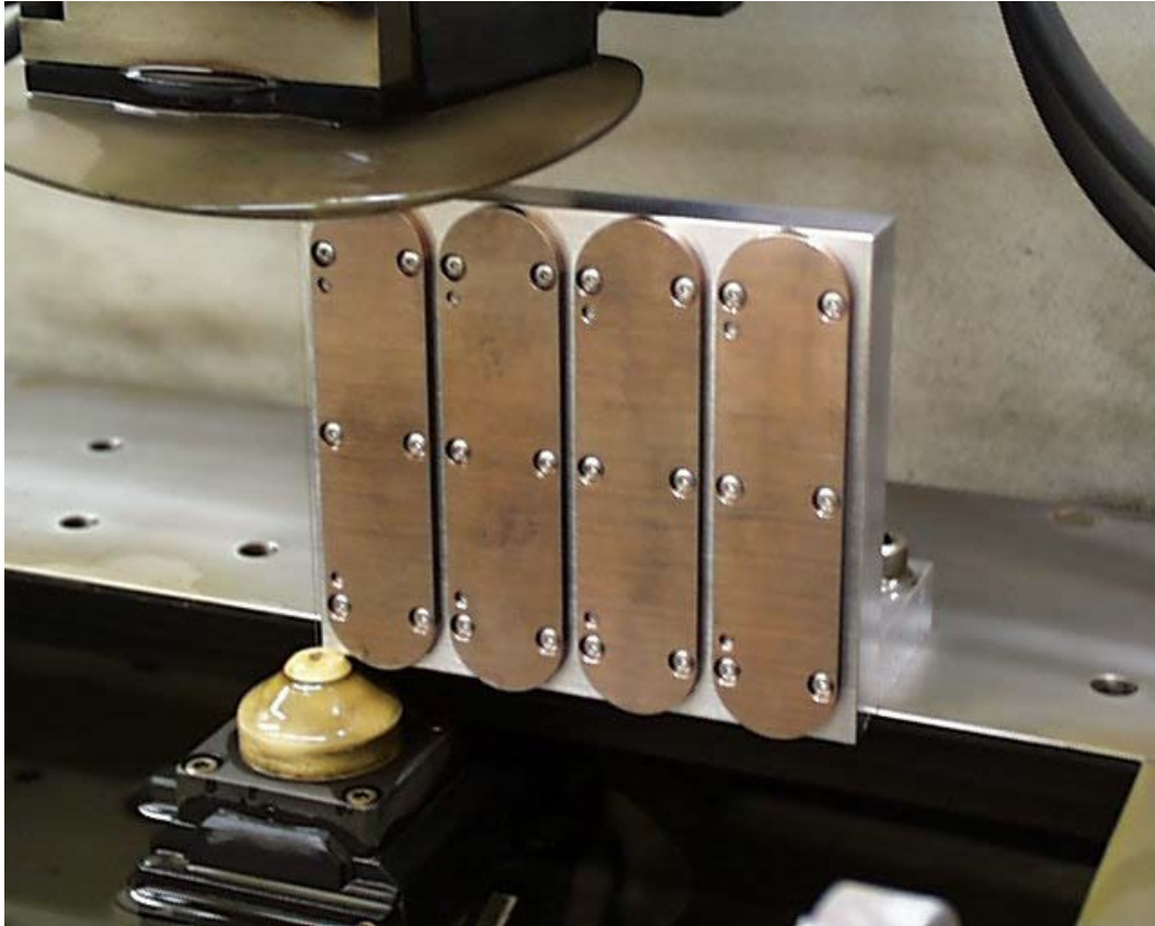
Figure 2.10 EDM set up for groove rail fabrication.
