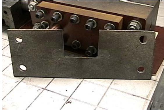
Figure 2.2 Ceramic spacer permits access from the top.
