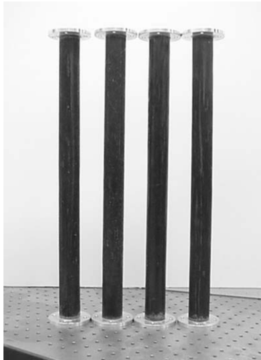
Figure 3.3 Four of the short beams with the base flanges in line and touching.
