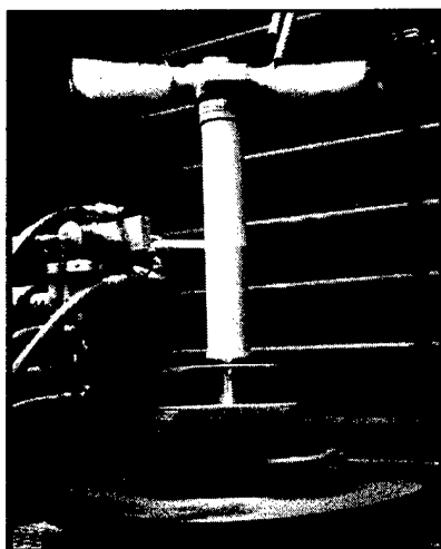
FIGURE 2 Application of HVOF WC/Co coating to Navy P-3 main landing gear cylinder.
