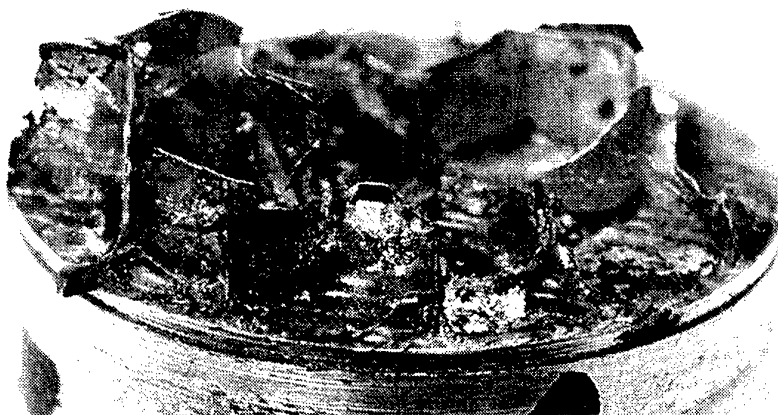
Figure 28 Failure surface of the portable adhesion test stub taken from the Stab-Tip after immersion in 50°C ionised water for 13 months, indicating regions of core corrosion leading to core fracture.
