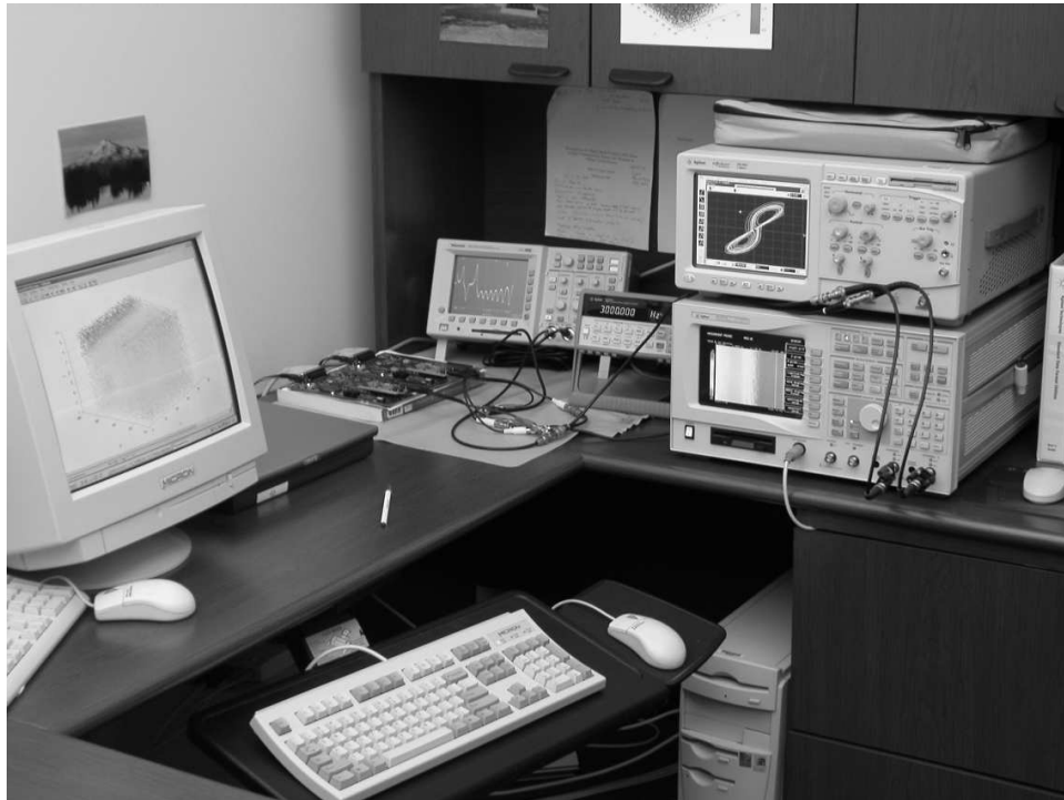
Figure 7.5: Hardware development station. Shown here: one of three computers used to conduct simulations and program or control the DSK devices, the two DSK boards with integrated 'C6711 DSPs, two digital dual-channel oscilloscopes, and a Vector Signal Analyzer. The later device measures characteristics of our system in the frequency domain.
