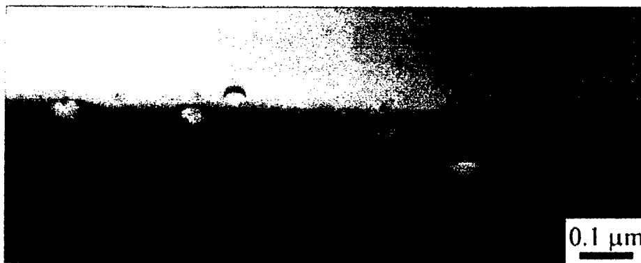
Transmission Electron micrograph of bonded interface
