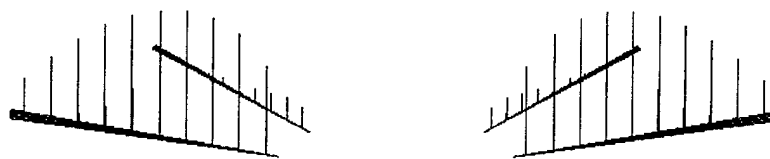
Figure 11: Aircraft Lift Distribution from Vortex-Lattice Solution
