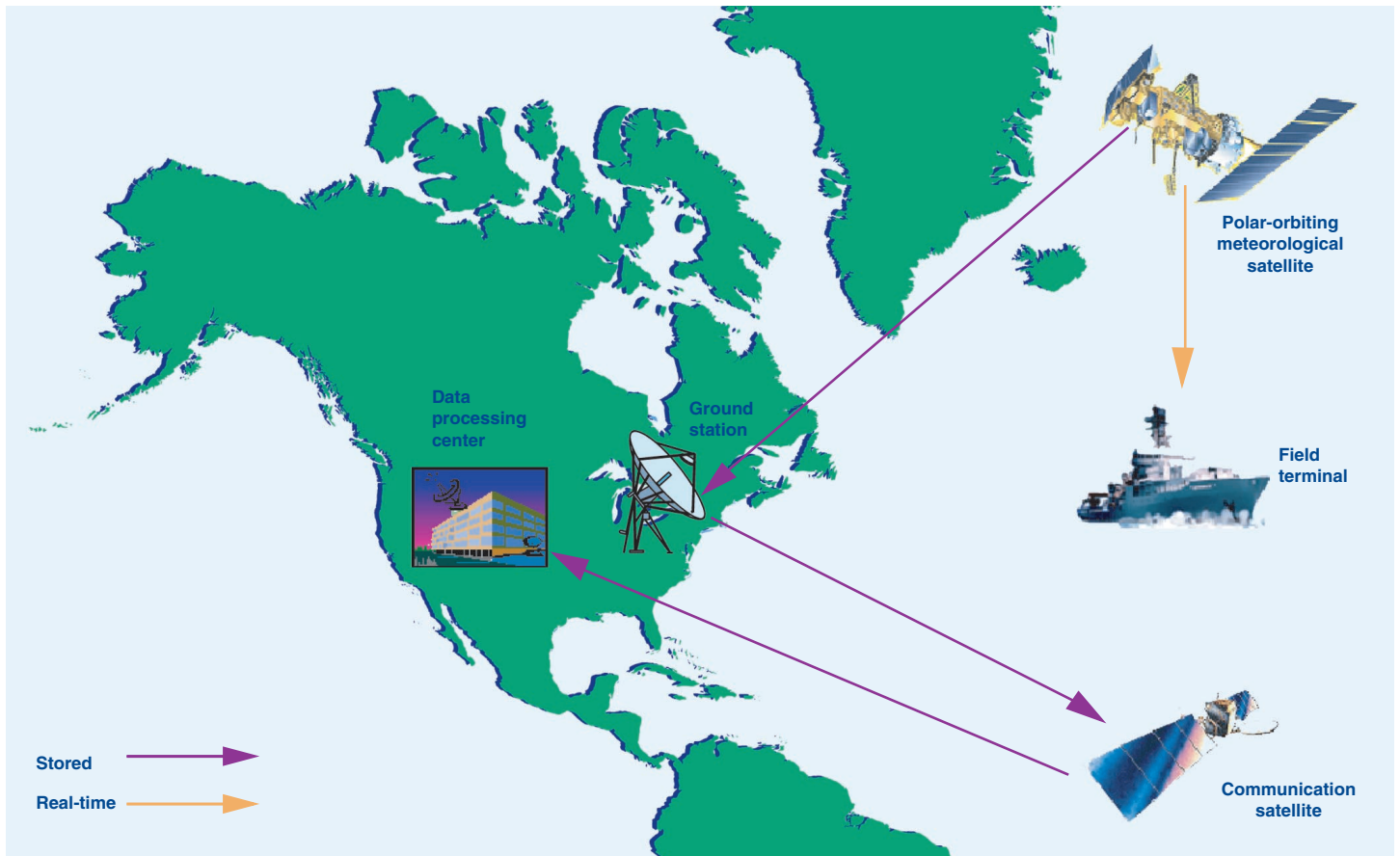
Figure 2: Generic Data Relay Pattern for the Polar Meteorological Satellite System
