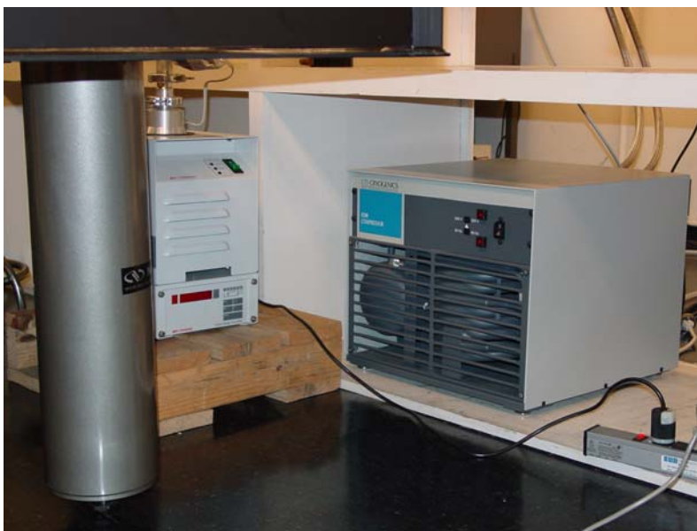
Figure 2.5 8200 Compressor is shown to the right of the digital photo, while the Turbopump is visible to the left.
