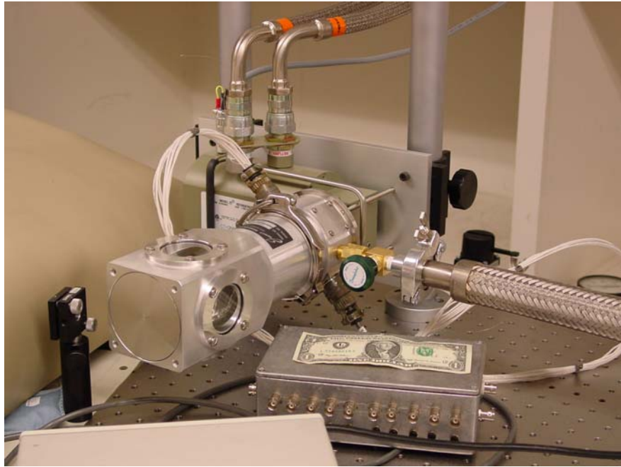
Figure 2.4 Close in digital photograph of the cold head and Model 22 Refrigerator. Helium lines are visible at the top and run to the compressor; the wider, woven tube at the right runs to the turbopump; the “bus” with one dollar bill included for scale is in the foreground.
