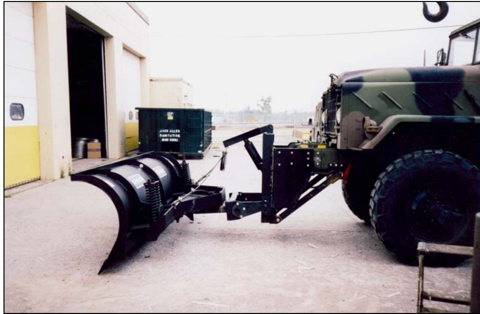
Figure 13. The 5-ton truck snowplow is manually reversible and hydraulically operated, 11 feet wide and 36 inches high. Note the hydraulic ram cylinder as compared to the 1943 jeep shown in Figure 1. The snowplow and its mount puts the snowplow nearly eight feet out in front. Plow guides are a necessity as an aide to the driver.
