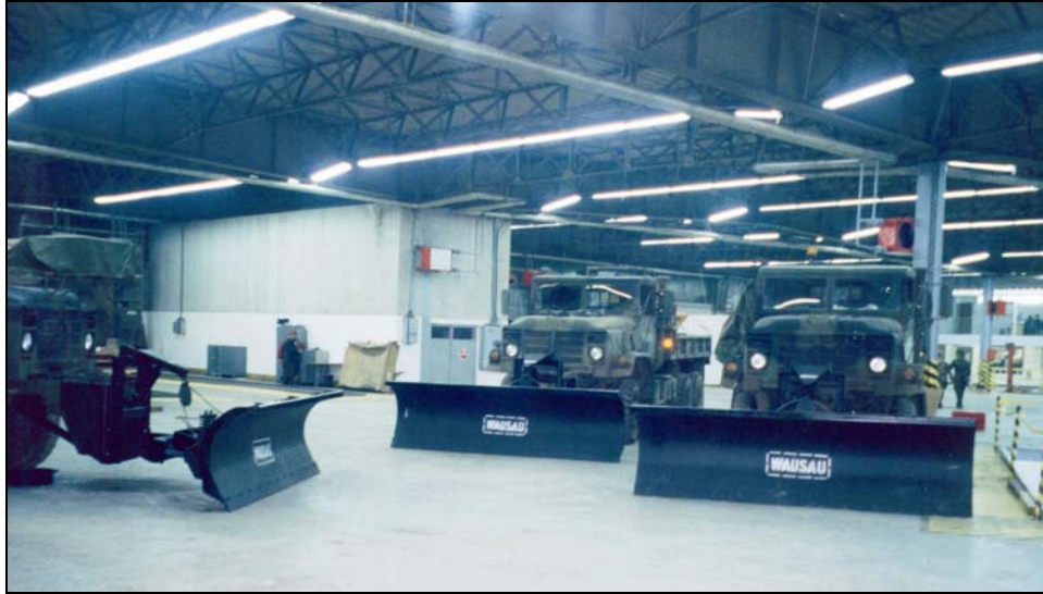
Figure 14. Heavy-duty “Wausau” brand Schmidt snowplows being mounted on 5-ton trucks in Kosovo for use by U.S. Army Kosovo Forces (KFOR). There are five of these plows in Kosovo.
