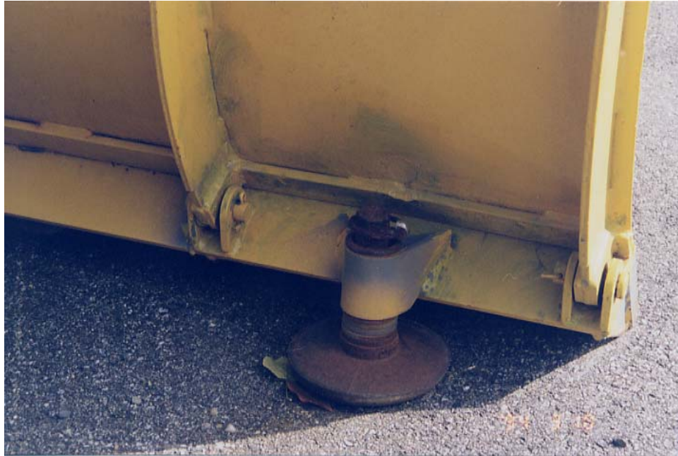
Figure 10. HMMWV snowplow with mushroom installed incorrectly. The shoe should be installed with sufficient spacer rings between it and the mounting bracket that permits the bottom of the shoe to be at the same level as the plow's cutting edge. Excess spacers should be tied on a string or wire and stowed in the vehicle; they should not be installed on the shoe shaft above the bracket as shown here. Doing so prevents the shoe from sliding on the shaft if the trip edge is deployed, thus causing the shaft to hit the back of the plow and eventually punching a hole in it.
