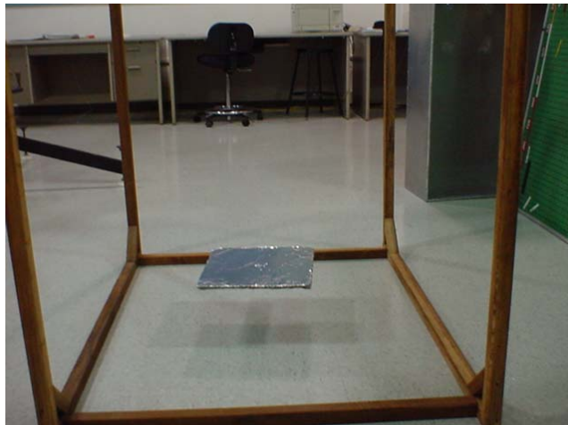
Figure 13. Wooden apparatus support for the impact hammer test
