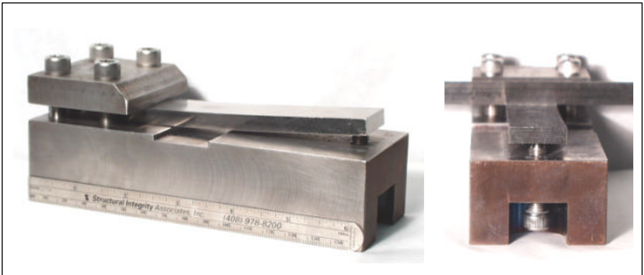
Figure 2. Loading fixture with compressive stress applied to a specimen.
