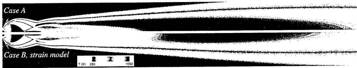
Figure 4.10. Comparison of temperature contours at 30 km for Case A (top) and Case B using the strain extinction overlay technique (bottom). The streamwise axial coordinate has been scaled.
