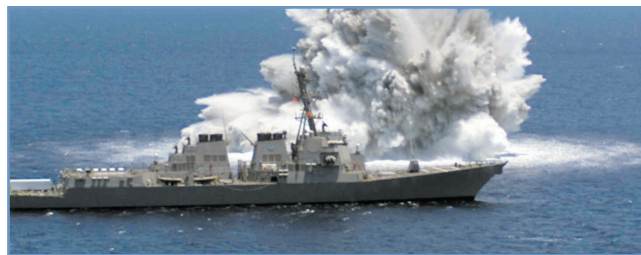
Figure 3. WINSTON S. CHURCHILL (DDG 81) Shock Trial
