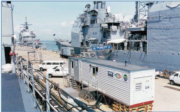
Figure 2. AMTS (in-tank membrane system) pier-side demonstration system trailer.
