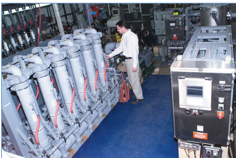
Figure 6. Laboratory checkout of the prototype 50 gpm oily waste membrane system.
