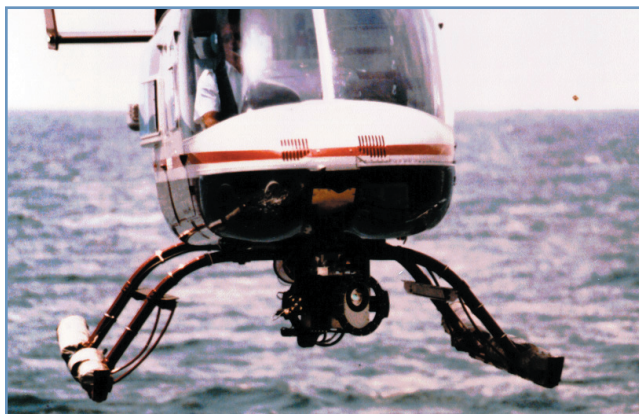
Figure 2. Helicopter-based radiometric signature measurement system.
