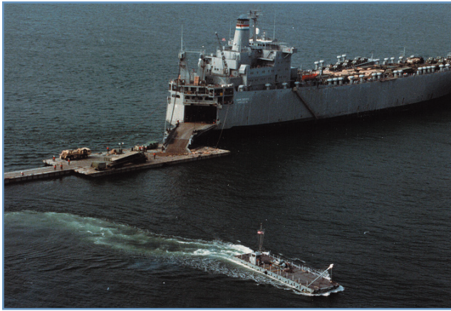
Figure 2. RO/RO ship discharging to lighters via discharge facility.
