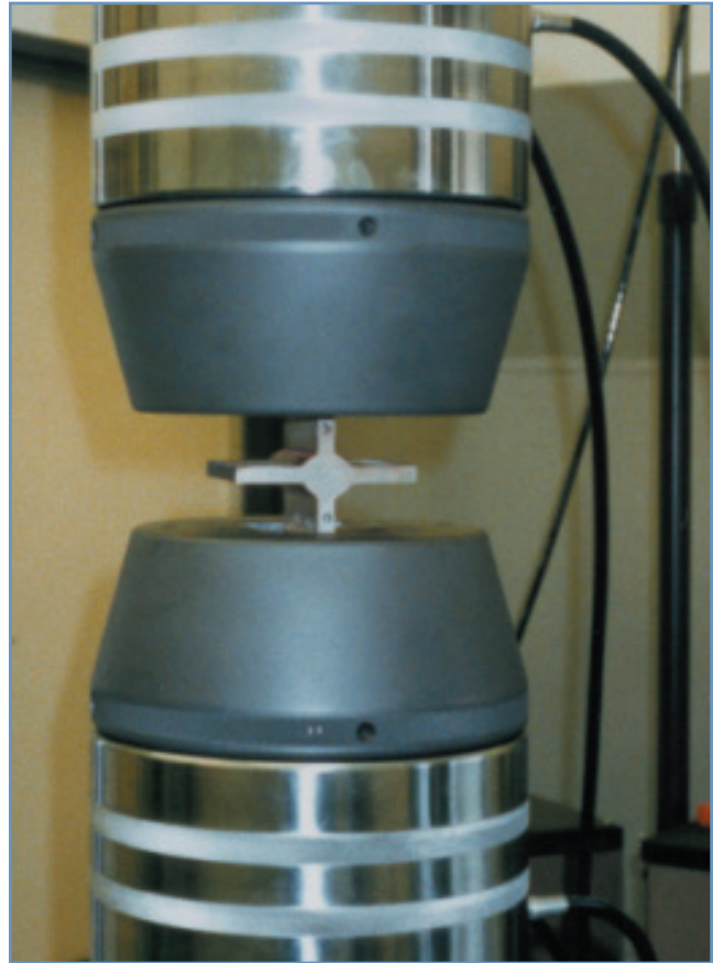
Figure 4. ADH fatigue specimen under test
