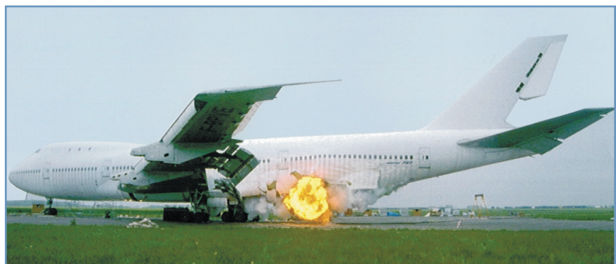
Figure 1. Explosive testing of a pressurized B747 aircraft at Bruntingthorpe, England, in May 1997.
