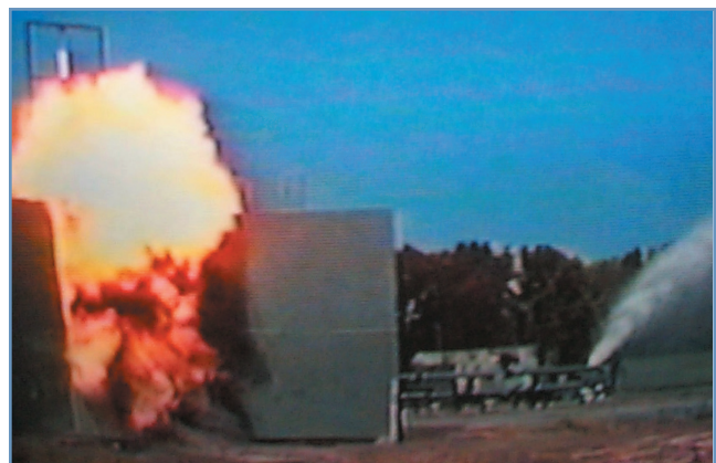
Figure 7. Automated fire main system demonstration with service loads activated.
