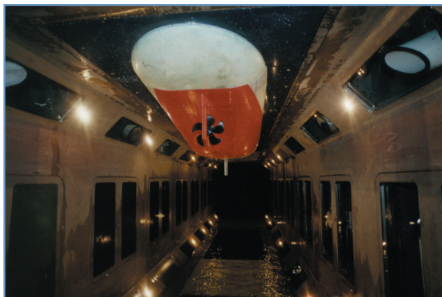
Propeller cavitation tests in NSWCCD's Large Cavitation Channel (LCC), Memphis Tenn.
