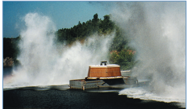
Figure 7. Target Acquisition System platform shock test.
