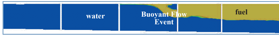
Figure 2. A buoyant flow event in a longitudinal section of Tank 5-300-2-F during a CFD refueling simulation at 1000 gpm.
