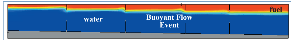
Figure 4. The positive effect (of adding 6 in. holes) in limiting a buoyant flow event in Tank 5-300-2-F during an SFST CFD refueling simulation at 1000 gpm.
