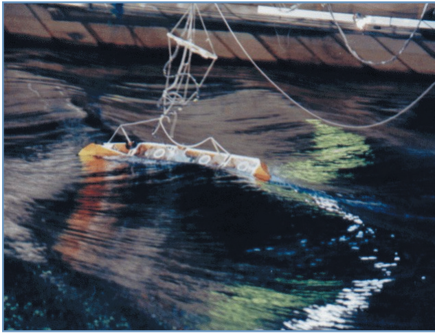
Figure 1. Capsize model test in NSWCCD Maneuvering and Seakeeping Basin.
