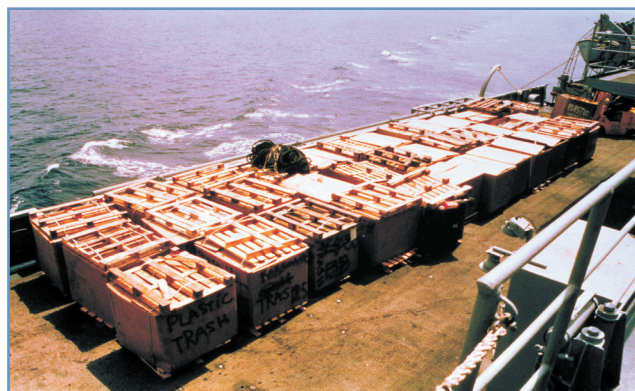
Figure 1. Photograph of tri-wall boxes used to contain the daily solid waste typically generated by a NIMITZ-Class aircraft carrier.
