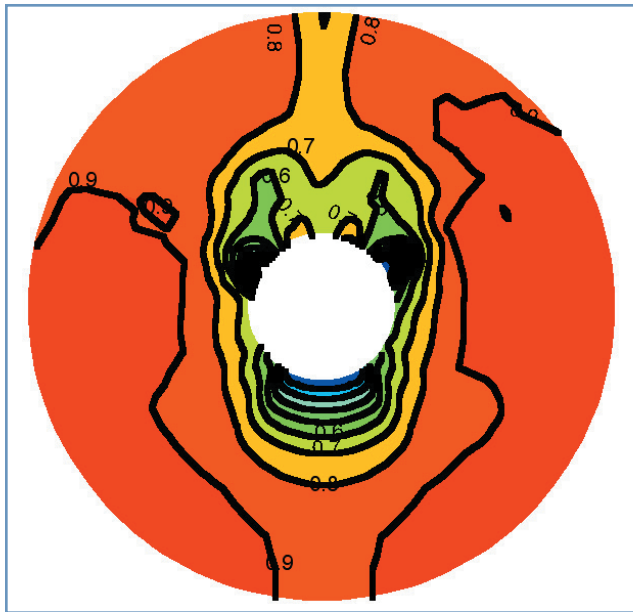
Figure 1. FRV-40 nominal wake, axial velocity contours.
