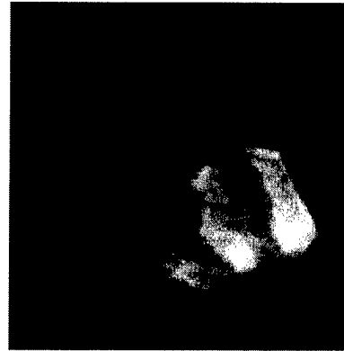
Figure 7: PMRI gradient echo image of a piece of bacon, demonstrating conventional fat-tissue image contrast. The matrix size was 64x64, 5 cm FOV, 780x780 \mu\text{m} in-plane resolution, 23.6 ms effective echo time, no averages, and a total imaging time of 30.1 s. No slice select was applied because the bacon slice was only about 4 mm thick. The polarizing pulse was applied at an amplitude of 0.55 T for 200 ms, allowing for T_1 image weighting. The fat is clearly brighter than the muscle.
