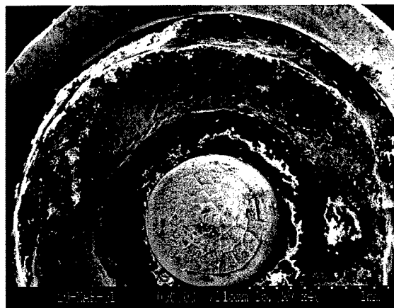
Figure 4. Propellant surface of 3.6 mm diameter micro-PPT
