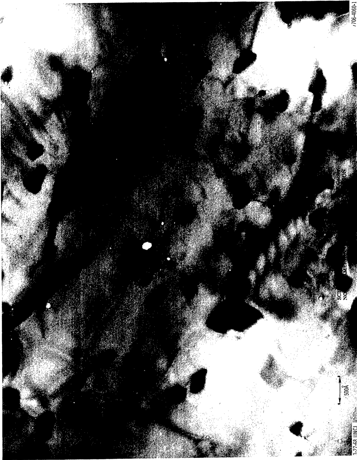
Figure 9a. Transmission Electron Micrograph Showing Helium Bubbles in Type 316 Stainless Steel Given Treatment 13 With 4 \times 10^{-5} Atom Fraction Helium Tested at 760^{\circ}\text{C}
