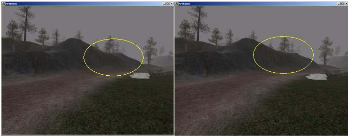
Figure 28. Apparent hysteresis. The left image showed a ridge low-resolution ridge being approached. The right image is the resulted swap to high resolution. The highlighted areas were the only differences noted as the entire hill was approached.
