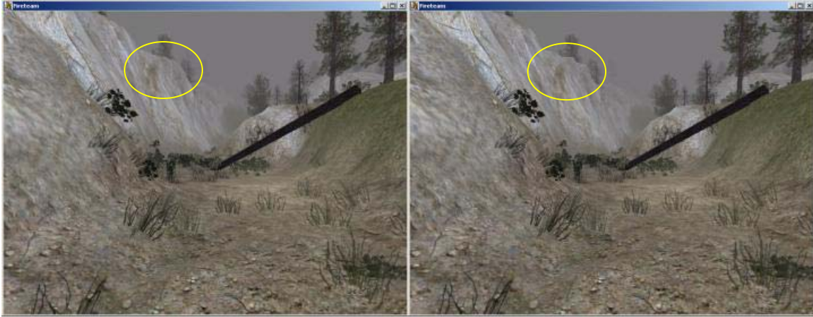
Figure 25. Close up of fractured terrain test. Left image is high resolution. Right image is high resolution close to the viewpoint and low resolution LOD distance away.
