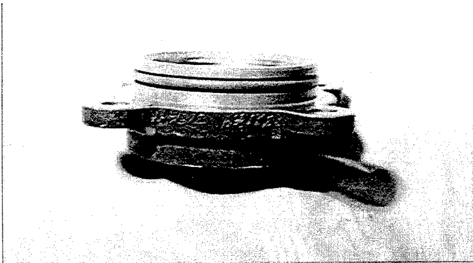
Figure 16 Typical O-Ring from Augmentor Fuel Pump Little wear evident.
