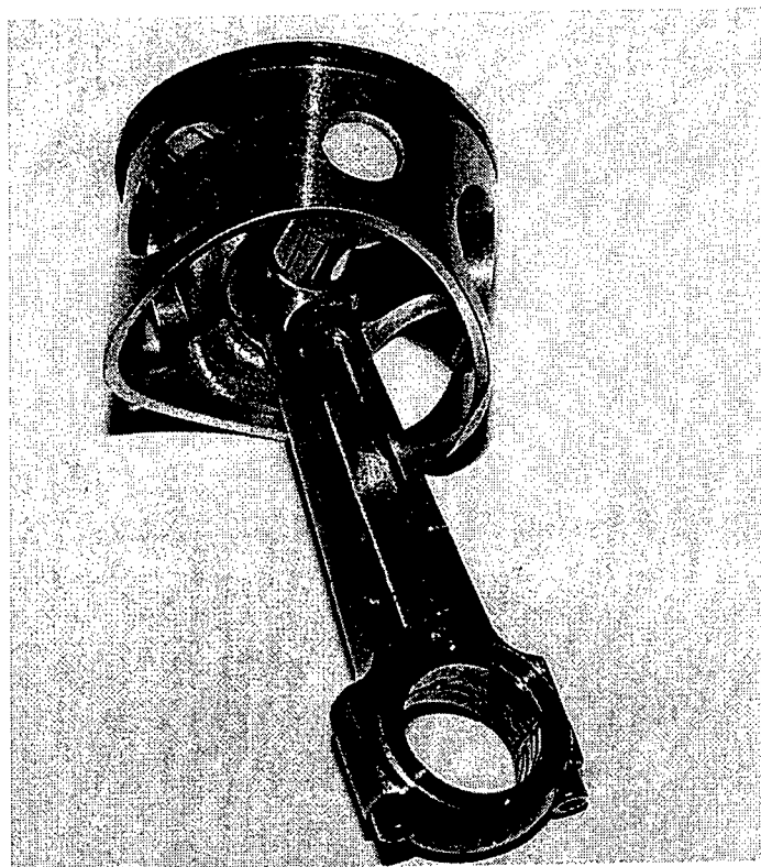
Figure 3.6: Assembly of a piston, piston ring and connecting rod.
