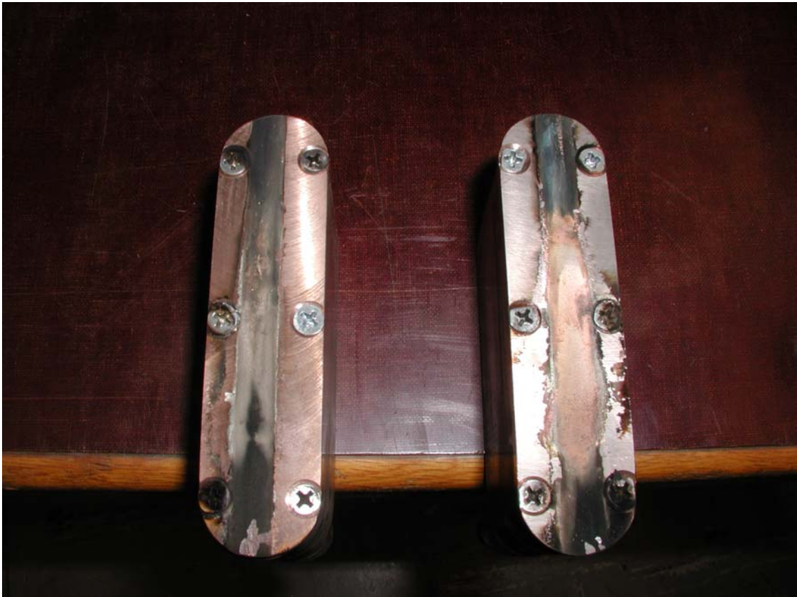
Figure 3. Erosion on rails from a shot with power supply capacitors charged to 5.5 kV
