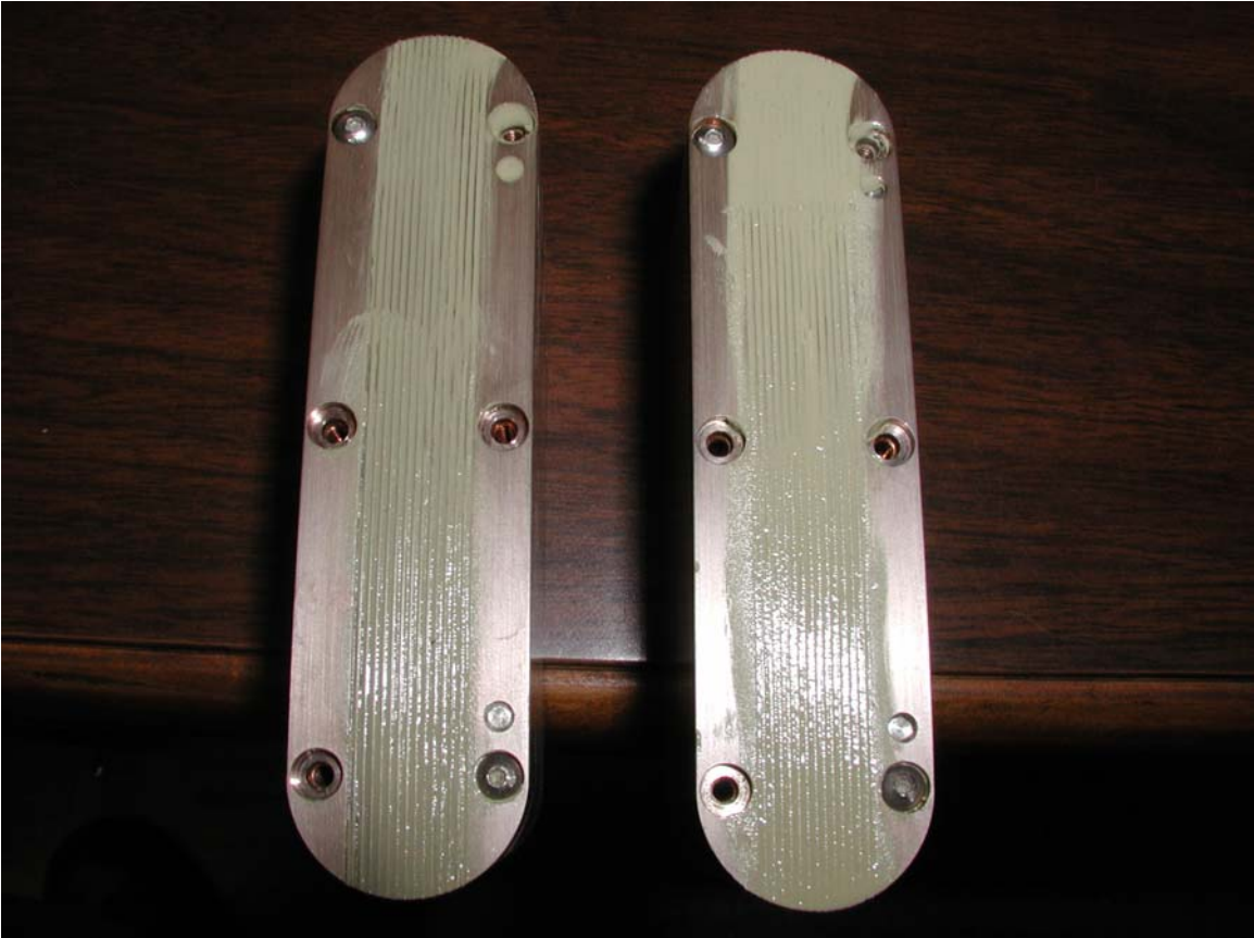
Figure 25. Rails coated with silver paste before firing
