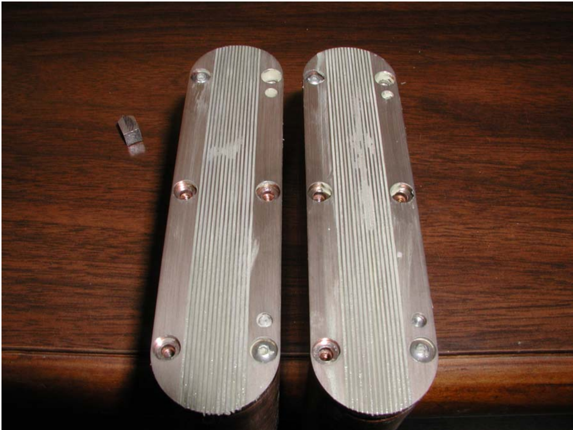
Figure 26. Projectile and rails coated with silver paste after shot
