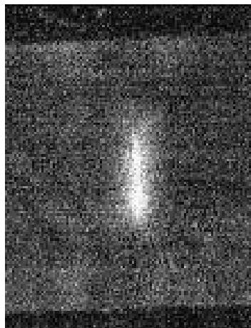
Figure 33. Thermal contrast generated on the fatigue crack specimen by sonic excitation.
