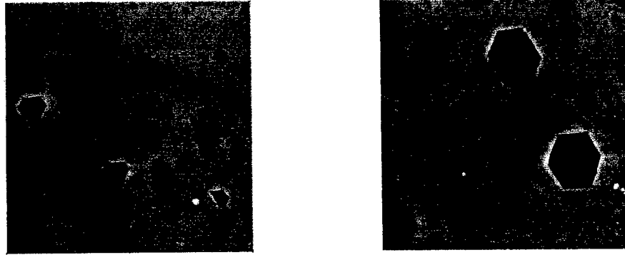
Figure 15: AFM images from the etched surfaces of sample C grown on a GaN/AlN buffer including an additional multiple quantum dot layers. The etching time is 6 minutes for (a) and 10 minutes for (b). The sizes of both images are 2 \times 2 \mu\text{m}^2 . The vertical scale for both images is 30 nm. Diameters of the three pits observed in image (a) are \sim 200 nm or less. Diameters of the two pits observed in image (b) are near 400 nm.
