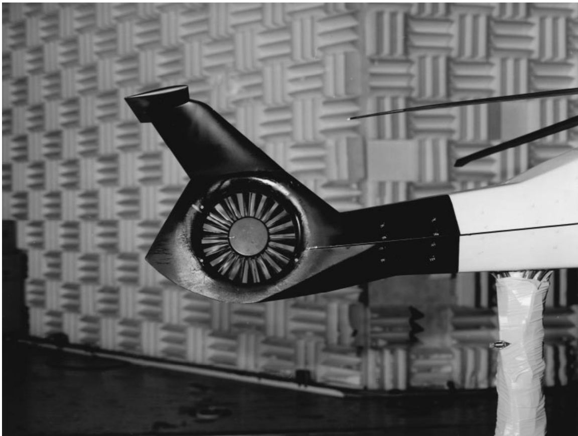
Figure 4. Tail fan configuration.
