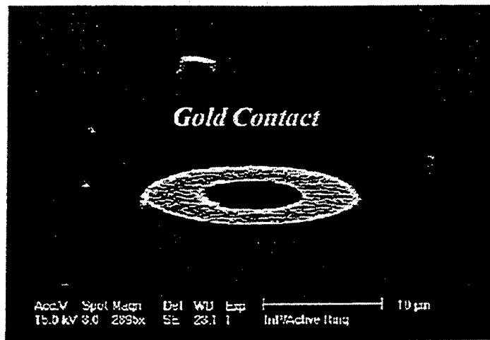
Figure 4.23 Gold Contact on the Top of the \mu -Ring
