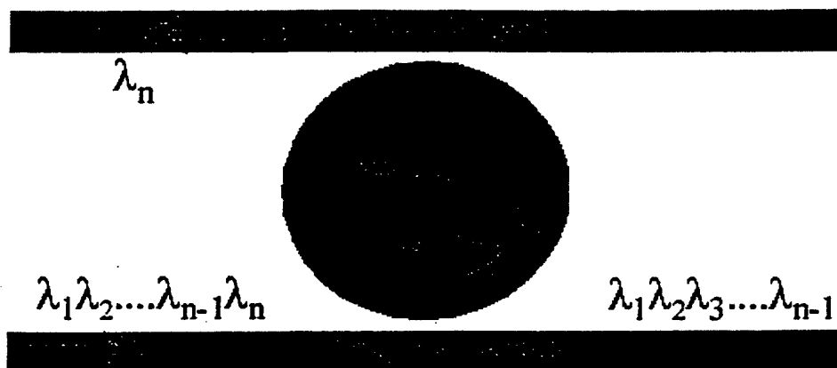
Figure 4.1 Schematic Diagram for Add/Drop Node with Single \mu -Disc Coupled to 2 Waveguides
