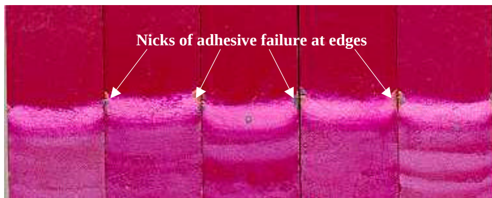
Figure 11: Failure Mode Exhibited by “Optimal” Nylon Pad Deoxidized Specimens Treated with Boegel-EPII and Tested at 140°F and 95-100% Relative Humidity
