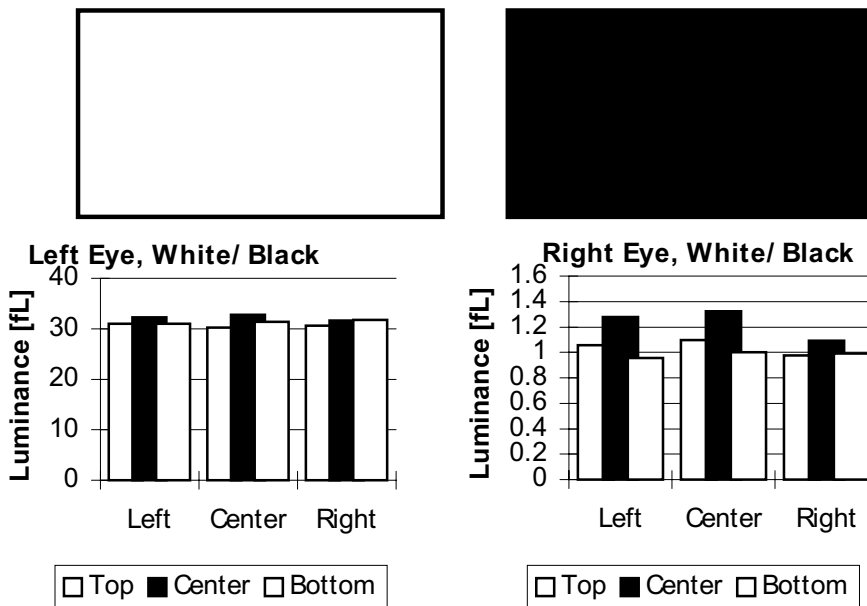
Fig.II.17-2. Spatial Uniformity of luminance in stereo mode when displaying white to the left eye while displaying black to the right eye.
