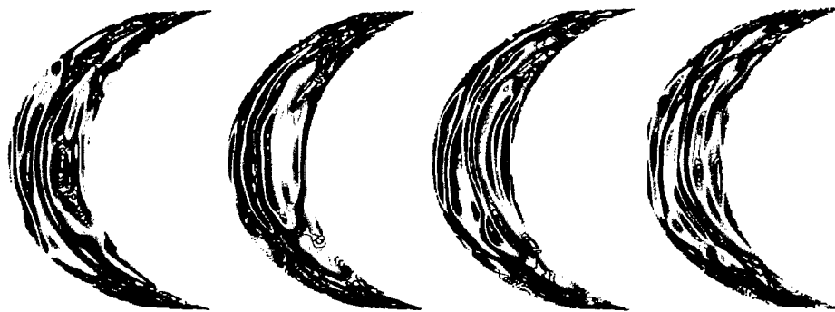
Figure 4: Snapshots of instantaneous heat transfer rate on a turbine blade leading edge surface.
