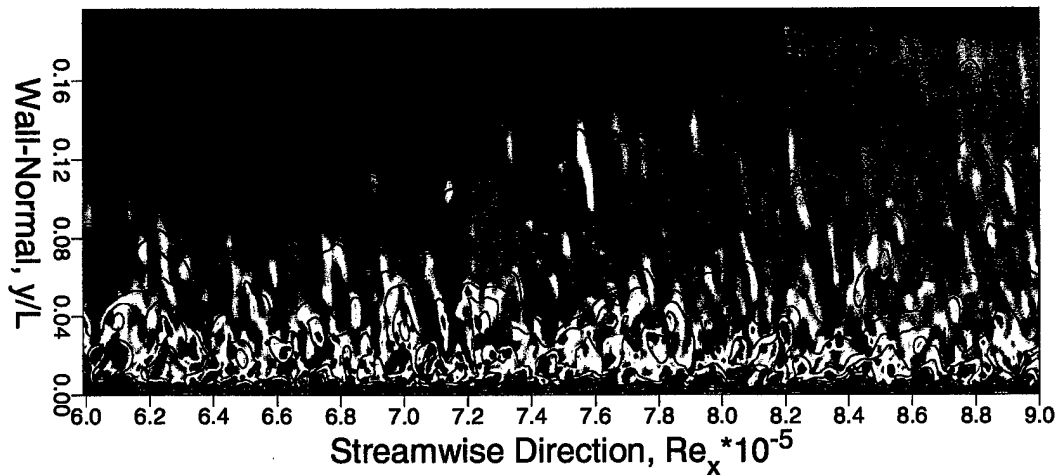
Figure 5.8 FSM applied to turbulent flat-plate boundary layer (incompressible). Color contours of instantaneous spanwise vorticity and isolines of instantaneous turbulent kinetic energy: FSM: \beta = 0.02 .
