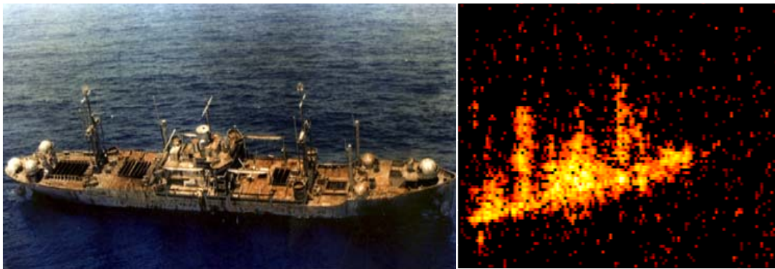
Figure 4. USS Crockett and AN/APS-137 ISAR Image of the USS Crockett.
