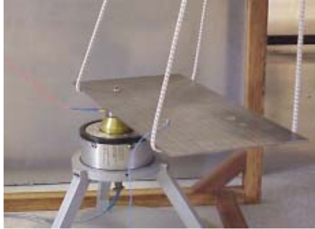
Figure 9. Flat plate test structure set up on Wilcoxon Generator
