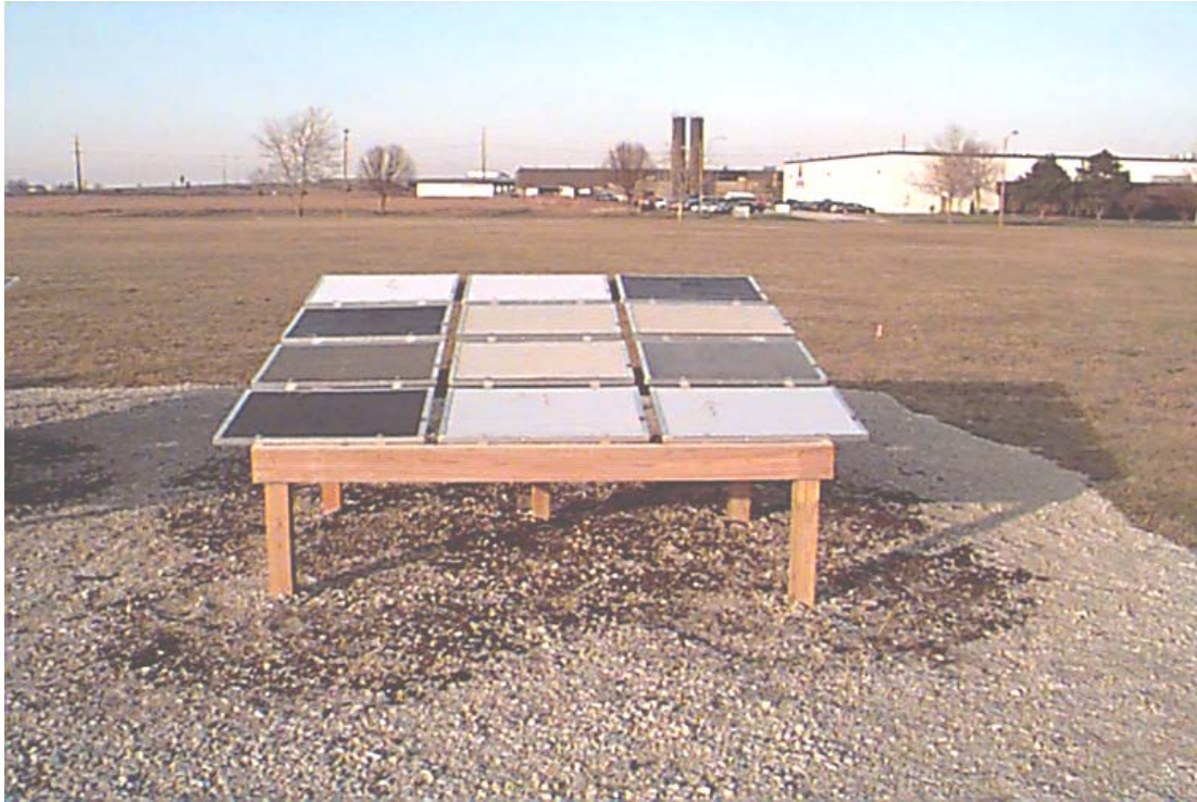
Figure 1. Outdoor exposure table with 12 samples at Champaign, IL weathering site.
