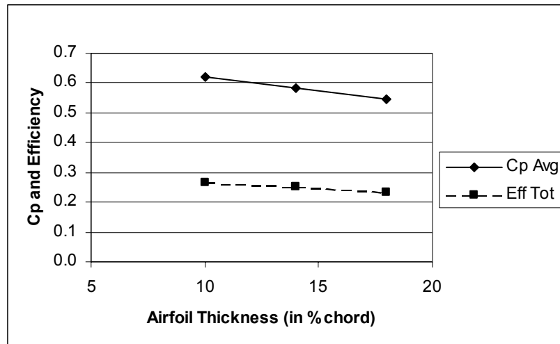
Figure 21. Effect of Airfoil Thickness on Power Production
