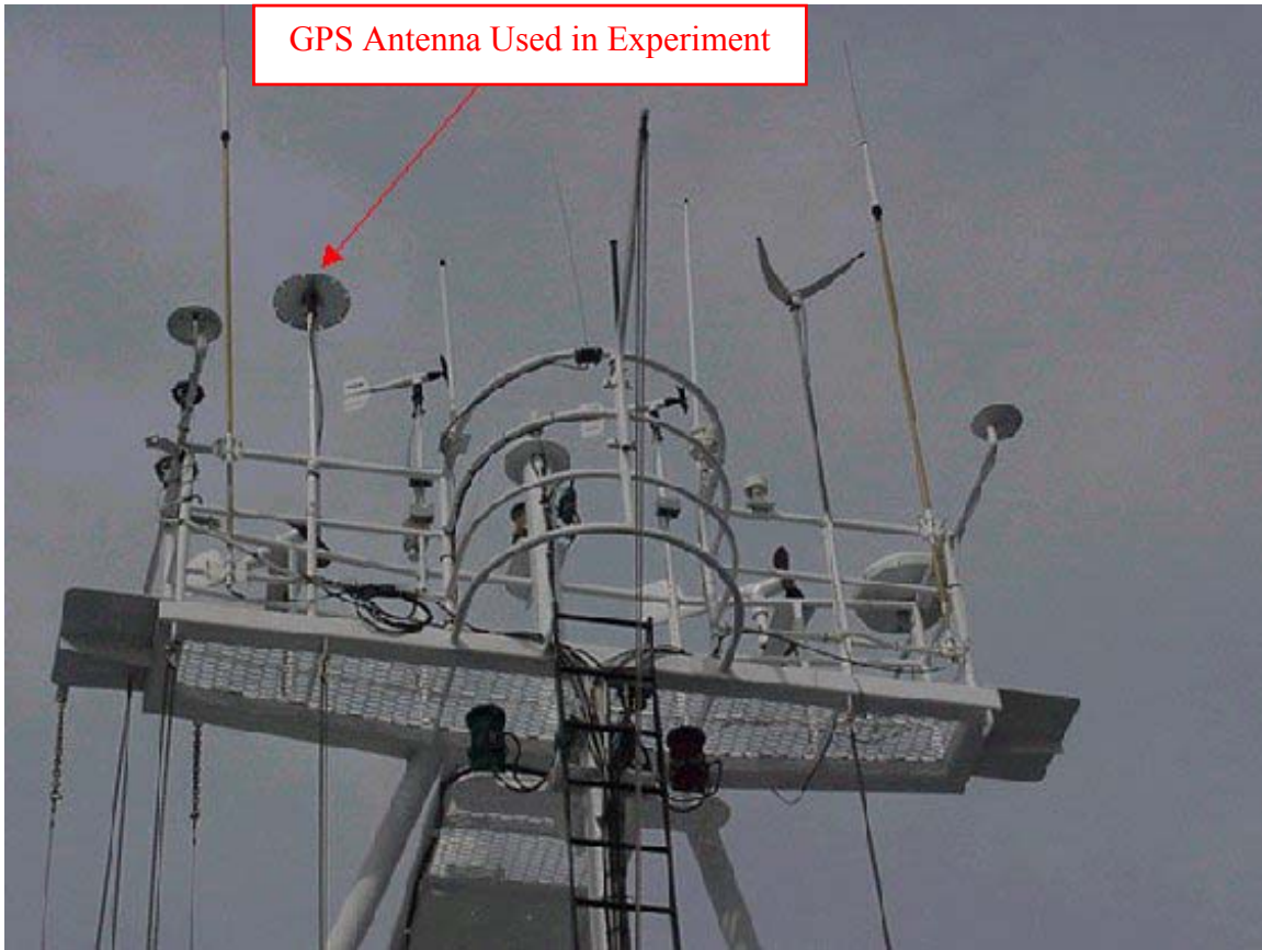
Figure 12 Arrangement of GPS Receiver Antenna on POINT SUR's Mast.
