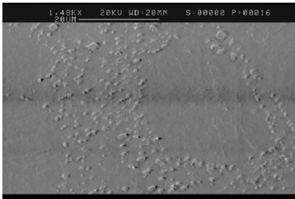
Figure 14. SEM photo of test sample after being aged 100 hours at 180C showing coarsened Ag 3 Sn particles.
