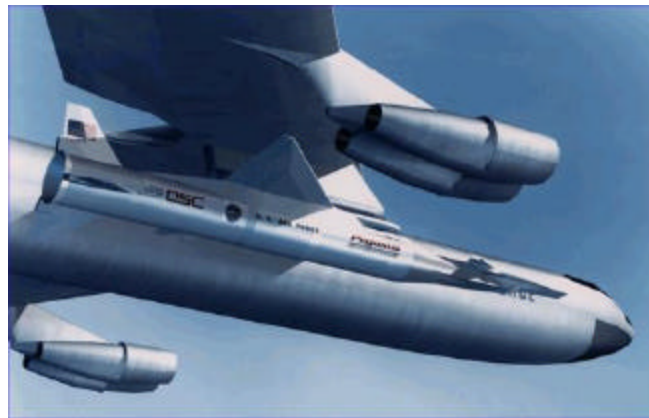
Figure 3.1 Pegasus/X-43 Launch Configuration
